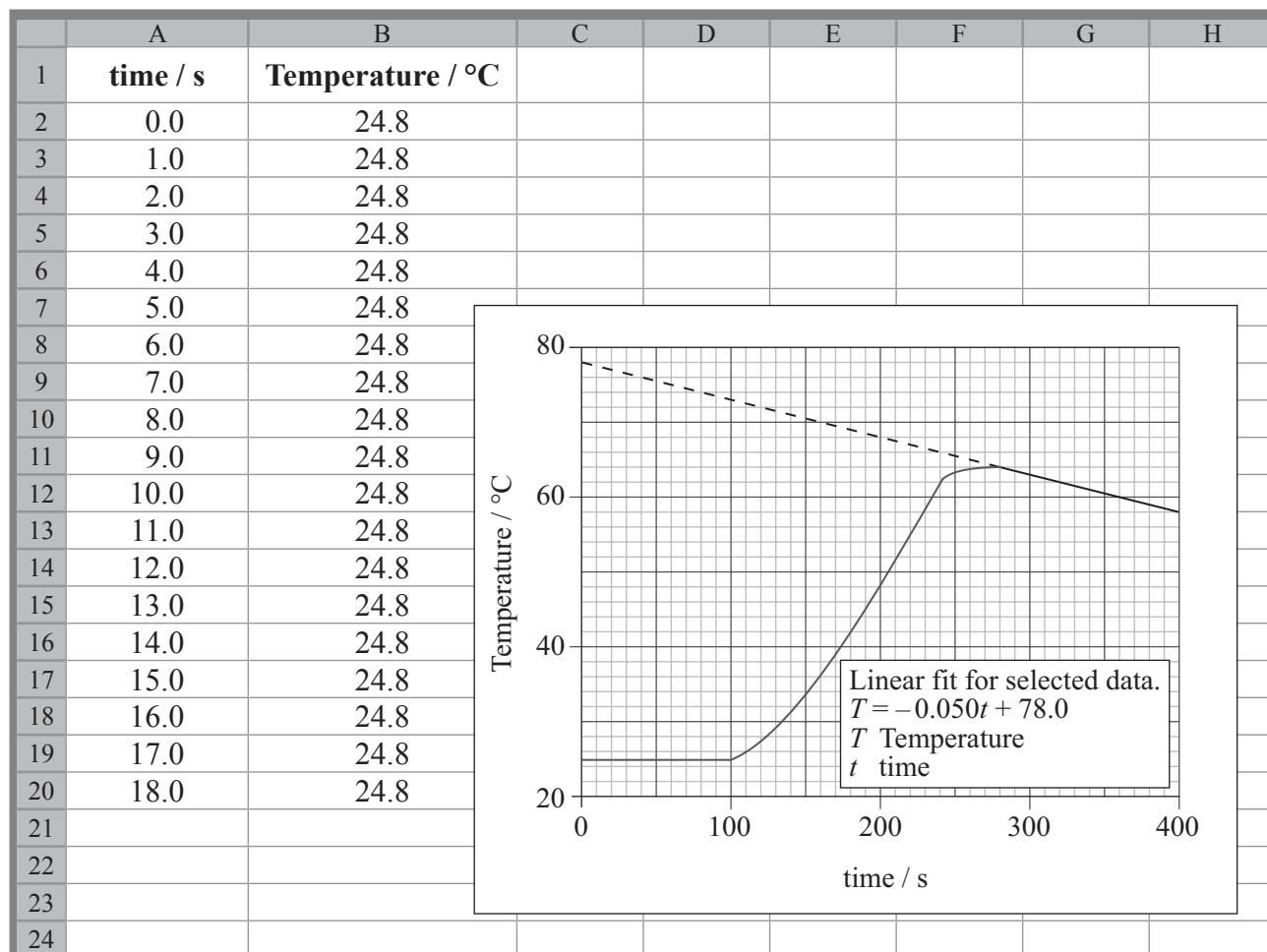
A straight line has been drawn through some of the data points. The equation for this line is given by the data logging software as
